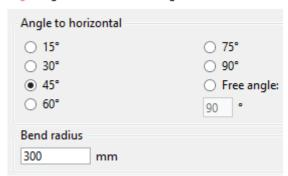
NOTE! The field is naturally disabled in case the tray series has fixed bend radiuses for vertical bends.
