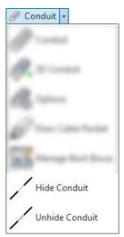
When using the "Hide Conduit" function, you need to show two points from a conduit segment and the segment will be hidden in the current view between those points by utilizing special union fittings and splitting the segment into pieces. The function continues as long as you press Esc.
