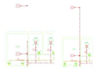
**Note:** When using the Mirror or Copy command of the Manipulate-tool the open ends aren't copied with the segments. But running MagiCAD's Check-function (MAGICHK) recreates them:
