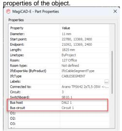
Bus circuit and Bus host attributes have been added to Object selection set under properties and all objects belonging to certain bus circuit or host can easily be filtered.
