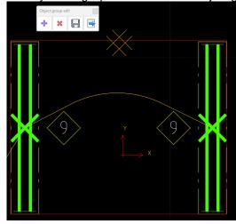
With Ungroup function, you can break any group instances and they will work as any installed object.
