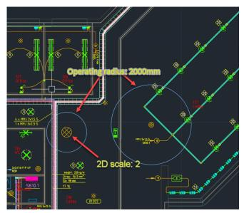
Now operation area is shown it's correct size regardless of the 2D scale of the symbol.
