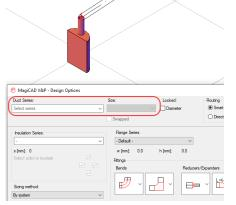
This has been fixed and drawing in the Z-direction is not allowed unless a duct series has been selected.
