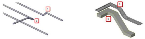
The second improvement is the possibility to use "Angle to horizontal" directly from the end of element, without being forced to draw a small piece first.
