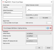
When using such circuit types in power circuits and creating switchboard schematic drawings from them, the circuit schematic templates are automatically stored/imported to the circuits in the drawings.
