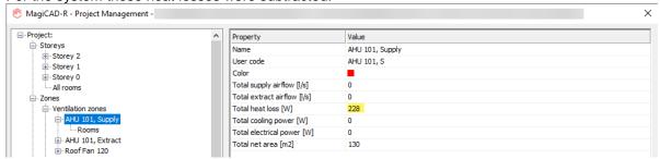
Now in MagiCAD 2023 the negative heat losses aren't subtracted in the system lists:
