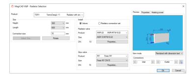
To be more logical and utilize the data in from the product with the data, the balancing limits are now read from the attached valve, if the radiator connection set is of a type without data, so the options are disabled:
