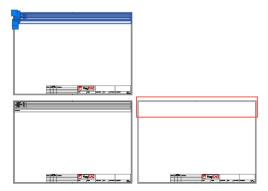
This issue was seen with BA-blocks where the P\_LTOP and P\_LBOT points of the frames' template were set at the very boundary, instead of like here within the page's boundaries, so in this example if P\_LBOT would have been set down to the left, where the arrow is pointing, then this issue would have occurred:
