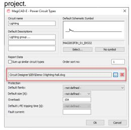
When using such circuit types in power circuits and creating switchboard schematic drawings from them, the circuit schematic templates are automatically stored/imported to the circuits in the drawings.
