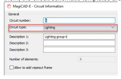
The templates can also be manually changed/assigned in switchboard schematics with the Edit Circuit function.
