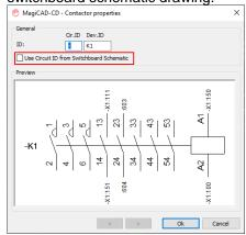
**Note!** Connected child parts cannot have "Use Circuit ID from Switchboard Schematic" active since they get their Circuit ID from the mother part.
